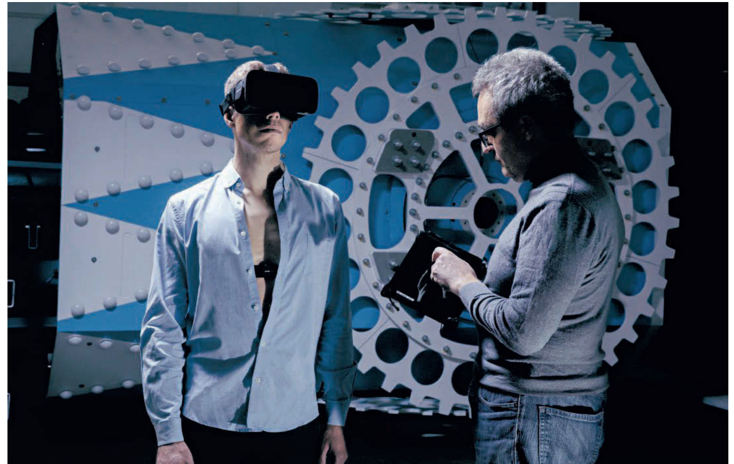
Above, biometric parameters of a user testing an augmented reality visor are measured through various sensors.
