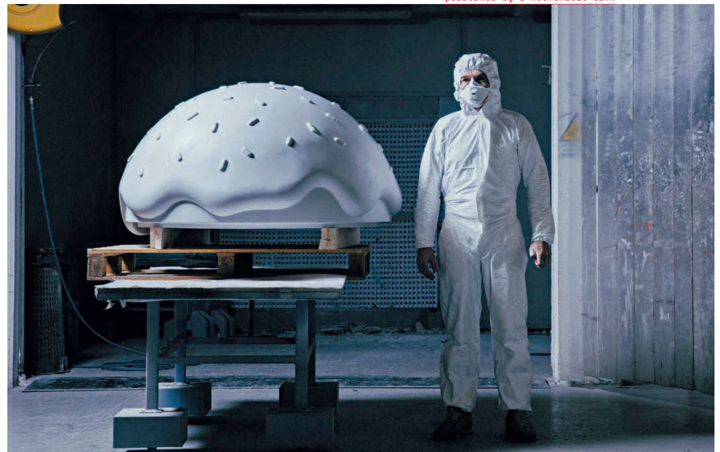
Below, a decorative fiberglass piece waiting to be hand refined after the milling performed by a mechanical arm.
